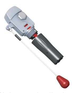
• Take the new automatic cartridge and screw onto the inflator head in a clockwise direction. Screw right up ensuring there is no gap between the cartridge and inflator head and then do up hand tight.
