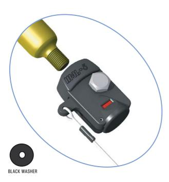
• Check that the cylinder sealing gasket in the end of the operating head has been correctly fitted, or replaced if necessary. Check the new CO<sub>2</sub> Cylinder has not been used and screw into the inflator body in a clockwise direction. Ensure the cylinder is screwed right down and do up hand tight.
